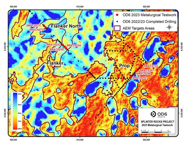
Figure 2: Splinter Rock Prop and Flanker metallurgical sample drill hole locations on AEM Model clay thickness
