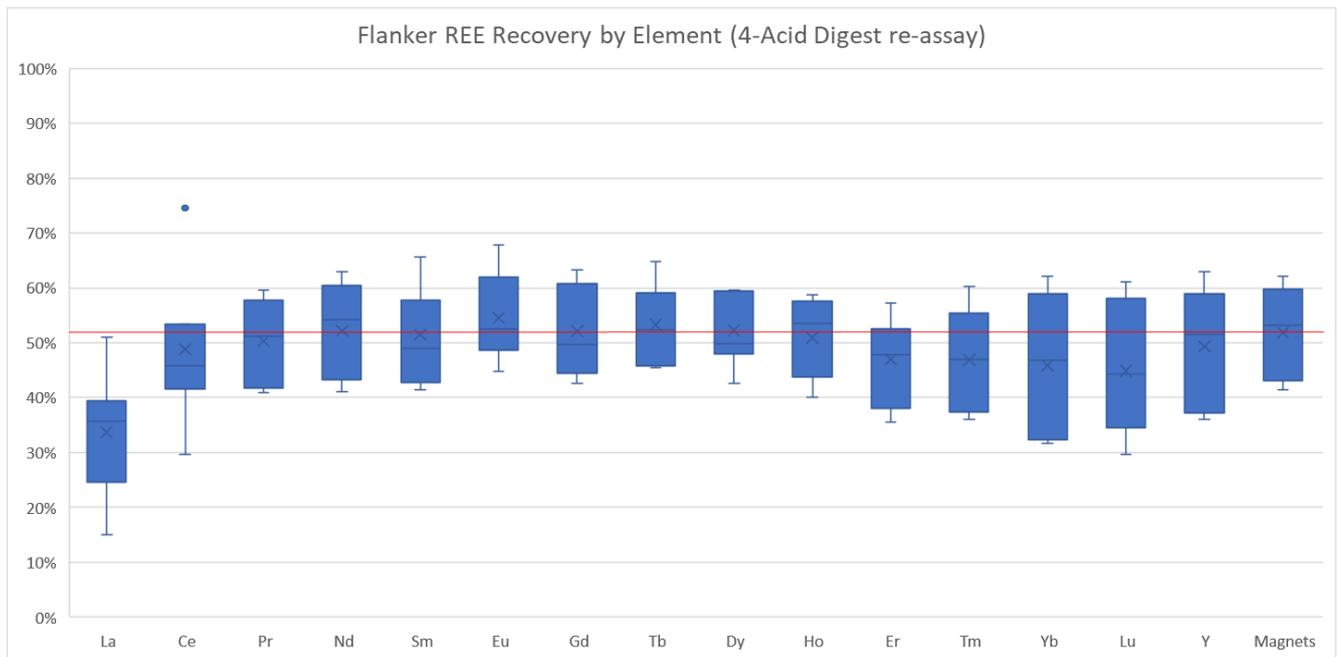
Figure 4: Flanker Prospect REE Recovery by Element (>40% MagREO recovery)
