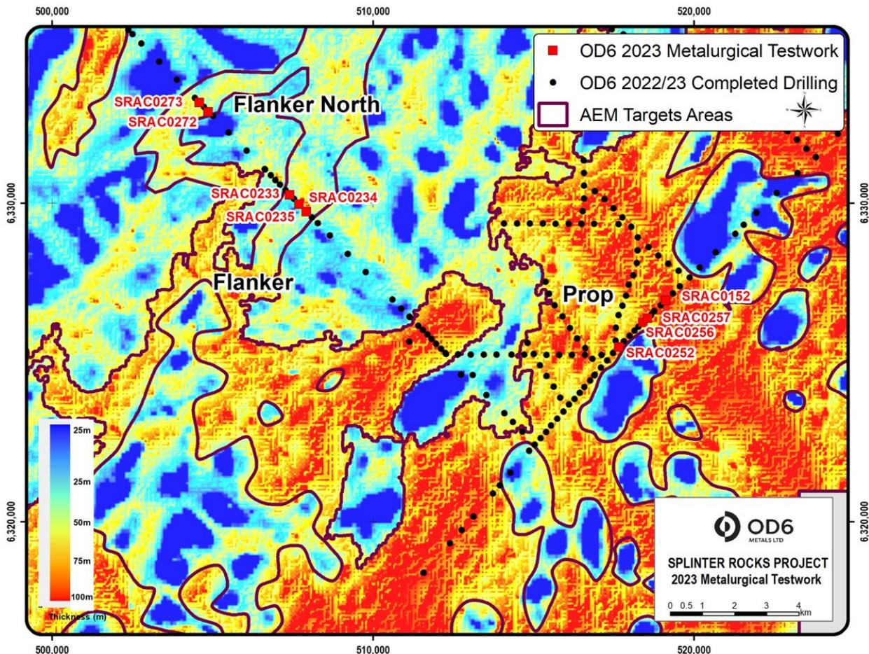
Figure 2: Splinter Rock Prop and Flanker metallurgical sample drill hole locations on AEM Model clay thickness
