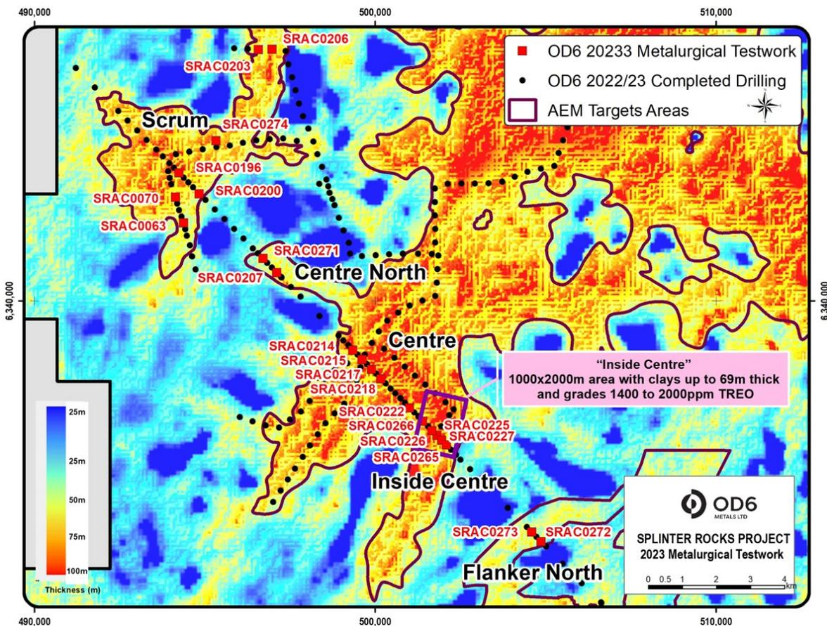
Figure 1: Splinter Rock Scrum and Centre metallurgical sample drill hole locations on AEM model clay thickness
