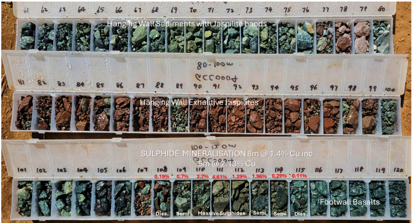
Figure 1: Chip Trays from Hole GC0004 showing the classic VMS stratigraphic succession from hanging wall sediments, jaspilite, disseminate to semi massive to massive sulphides to footwall basalts
