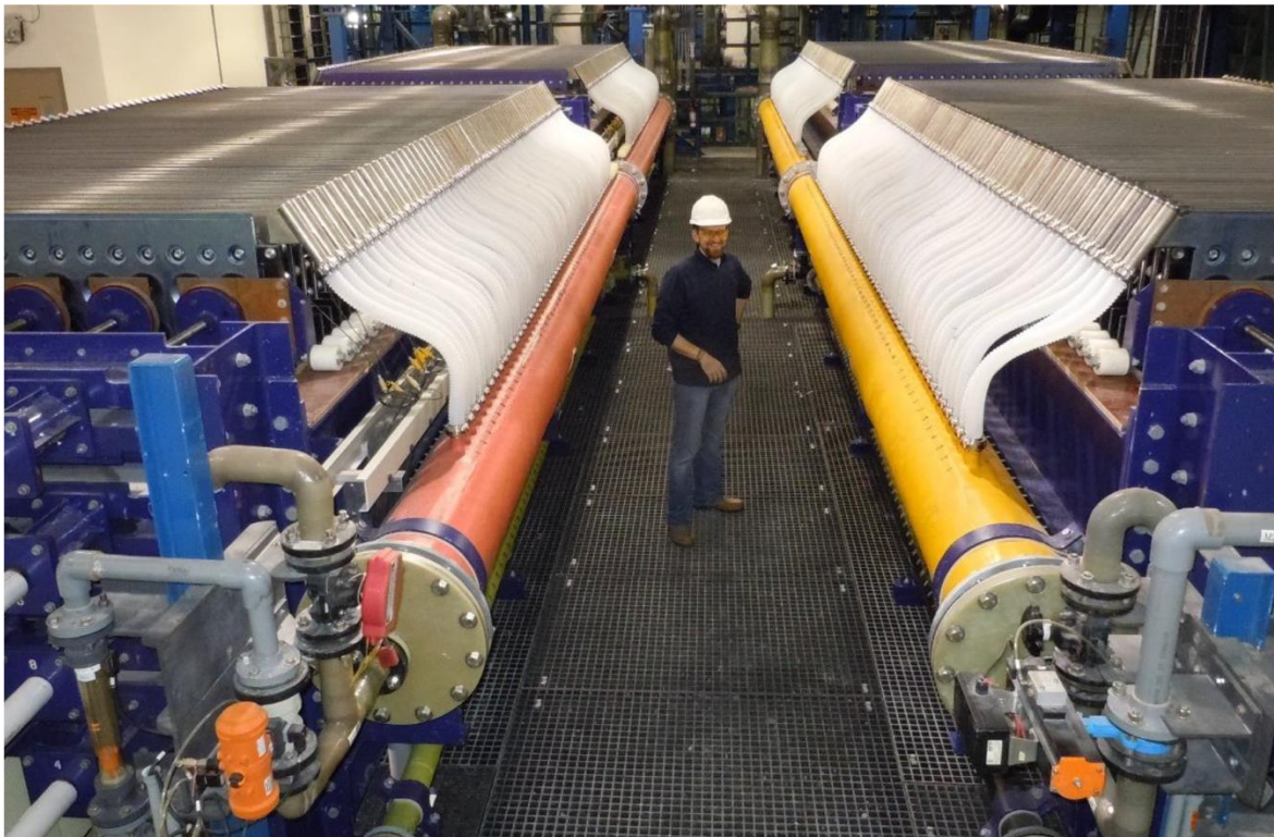
Figure 1: Example of two BICHLOR™ Electrolysers utilised to produce \text{H}_2 \text{ (g)} + \text{Cl}_2 \text{ (g)} + 2\text{NaOH (aq)}
